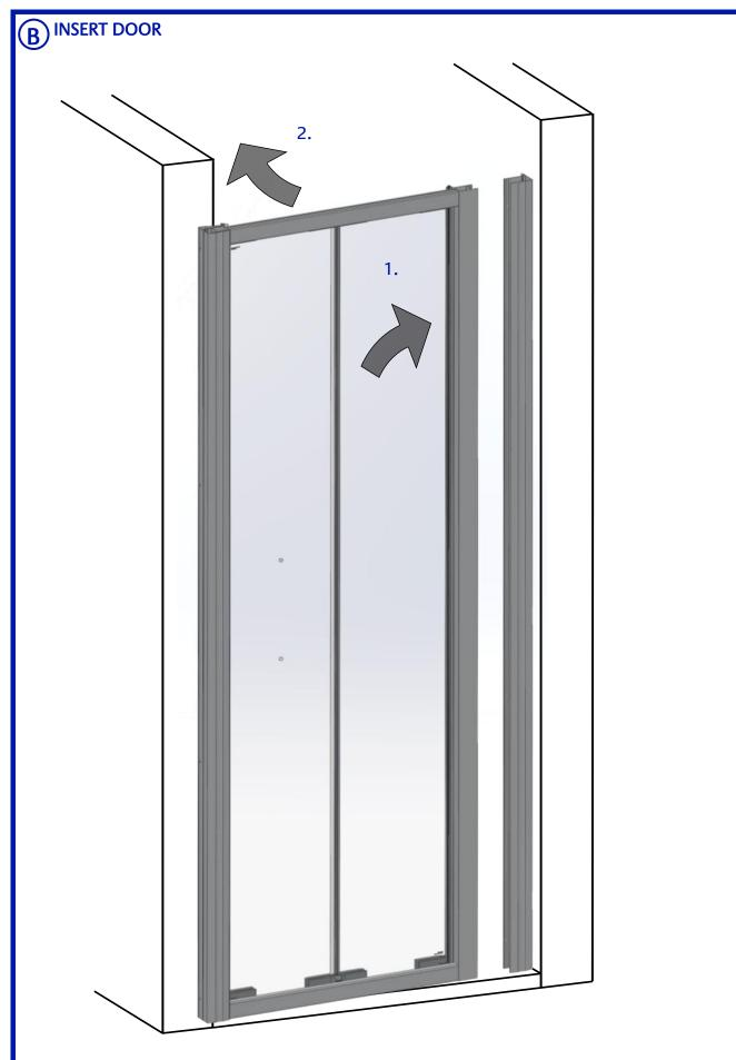
With 2nd wall profile fitted to frame:
