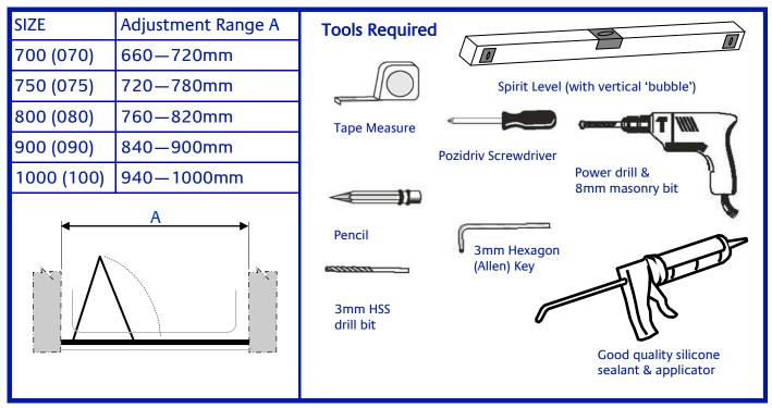
Lakes Coastline Bifold Door is fully reversible, so suitable for fitting with hinge to left or right hand side of enclosure. Ensure tray is correctly levelled & that all tray/wall joints are sealed & cured over entire length of tray sides (See - - - - Fig A) prior to fitting enclosure. DO NOT SEAL BASE / WALL EDGES UPTO A FITTED ENCLOSURE!
