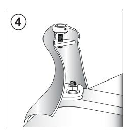
To secure the bath to the floor place a small amount of silicone under each foot where it meets the floor.
