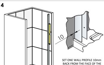
TRAY. MAKE SURE IT IS TRUE WITH A SPIRIT LEVEL, THEN MARK THROUGH THE FIXING HOLES WITH A PENCIL. REMOVE PROFILE THEN DRILL AND PLUG THE WALL (ITEM 26). NOW FIX THE WALL PROFILE IN PLACE USING ITEMS 24, 27\* & 28\*
