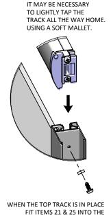
FIT ITEMS 21 & 25 INTO THE TOP HOLES (WHERE SHOWN) TO LOCK THE TRACK IN PLACE.
