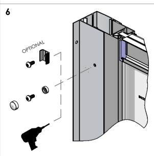
WHEN THE FRAME IS READY TO BE FIXED, DRILL THROUGH THE HOLES IN THE WALL PROFILE WITH A 3mm DRILL. (MAKE SURE YOU ONLY DRILL THROUGH ONE WALL THICKNESS) THEN FIX THE FRAME WITH ITEMS 25, 27\* & 28\*
