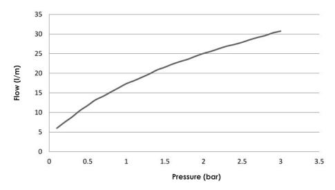
An SC50 Cartridge was placed in a standard body in order to record the above Pressure vs. Flow graph.
