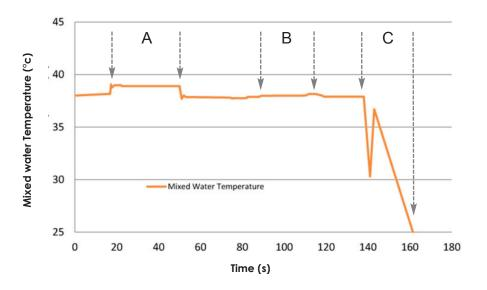
Note: This test was carried out using a standard body. The initial Hot and Cold inlet pressures were 3 bar.
