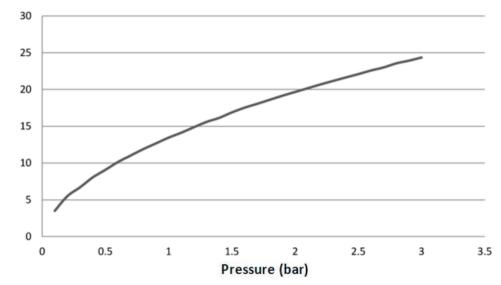
An SQ50 Cartridge was placed in a standard body in order to record the above Pressure vs. Flow graph.
