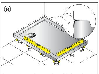
Ensure the 'easyseal' water sealing strip is flat to the wall. Place the tray into position and level both ways using the legs. After the tray has been levelled adjust all the inner feet to stabilise the tray. When level fix these legs to the floor with silicon sealant or 'no more nails' type adhesive.
