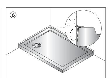
Ensure the 'easyseal' water sealing strip is flat to the wall. Place the shower tray onto the cement bed and apply gentle pressure with the palm of the hand to bed the tray into position.
