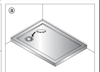
When shower tray is set remove the remainder of the protective plastic film and connect the waste pipe and check for leakage and water drainage.
