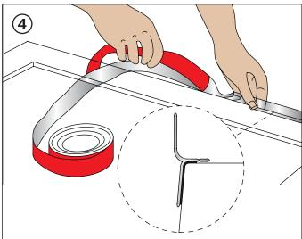
It is recommended that the 'easyseal' water sealing strip should be installed at the sides against wall. For the detailed installation method, please refer to the "Waterproof Sealing Strip instruction".
