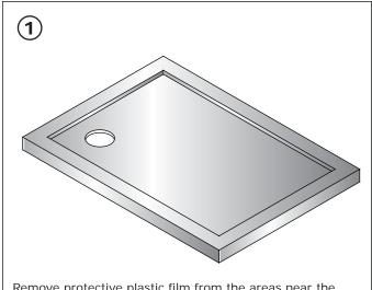
Remove protective plastic film from the areas near the waste and those sides of the tray which will be against a wall.
