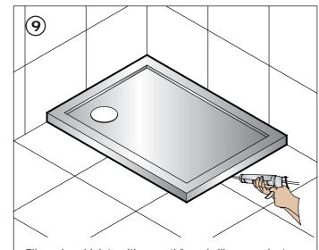
Tile and seal joints with an anti fungal silicone sealant and allow to set.
