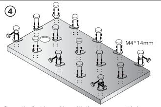
Screw the feet in position with the screws provided. Ensure that the foot that has two panel fixing rods attached, is placed in the corner where the panels will
