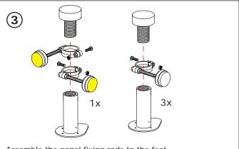
Assemble the panel fixing rods to the feet.
