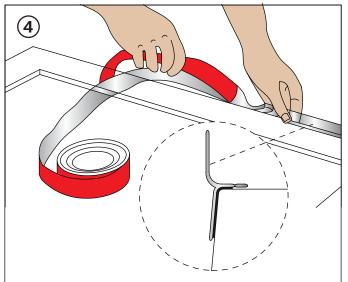
It is recommended that the 'easyseal' water sealing strip should be installed at the sides against wall.
