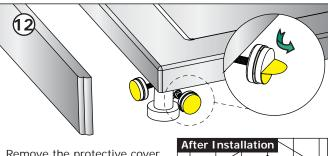
Remove the protective cover from the adhesive tape. First fix the rebated panel pushing it firmly on to the adhesive pads. Then fix the remaining panel in the same manner.
