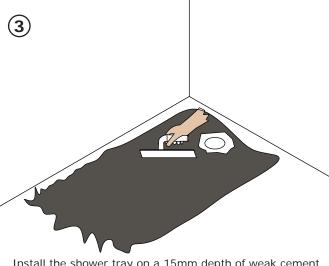
Install the shower tray on a 15mm depth of weak cement mix (sand/cement ratio 5:1). Tile adhesive can be used as an alternate to sand or cement.
