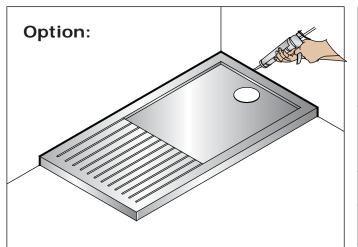
\* If the 'easyseal' water sealing strip is not installed, please seal joints between tray and wall with an anti fungal silicone sealant and allow to set.
