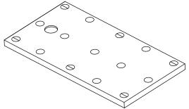
Turn the tray over and use the cardboard packaging as a protective mat. Note the circles that have been marked to should fix the feet with the panel fixing rod, but for the symbol  $\bigoplus$  you will only use four of these positions and the other two would be supplemented with the feet without the panel fixing rod.
