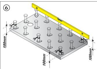
When all of the feet have been fitted the feet, the feet in the corner positions should be adjusted to 100mm.
