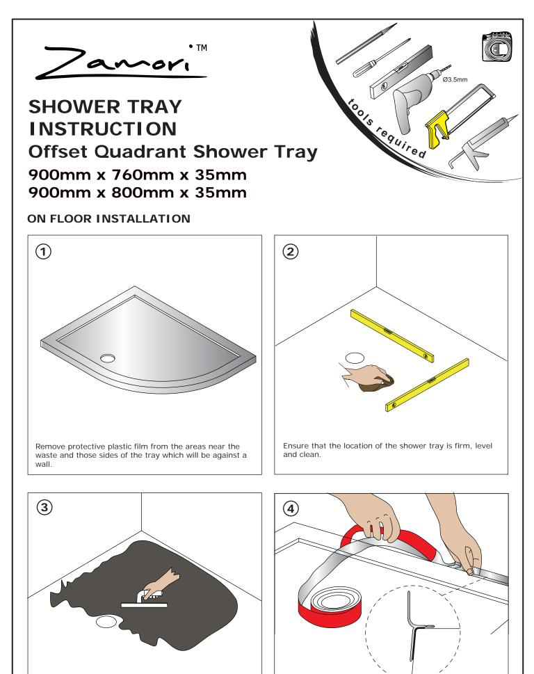
Install the shower tray on a 15mm depth of weak cement mix (sand/cement ratio 5:1). Tile adhesive can be used as an alternate to sand or cement.
