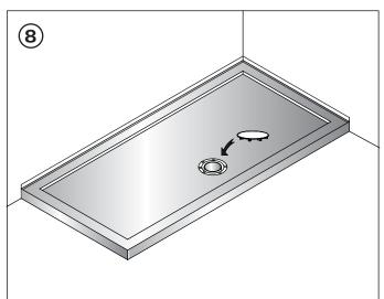
When shower tray is set remove the remainder of the protective plastic film and connect the waste pipe and check for leakage and water drainage.
