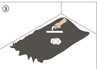
Install the shower tray on a 15mm depth of weak cement mix (sand/cement ratio 5:1). Tile adhesive can be used as an alternate to sand or cement.
