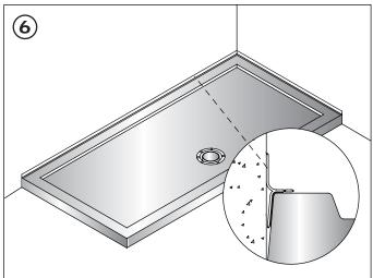
Ensure the 'easyseal' water sealing strip is flat to the wall. Place the shower tray onto the cement bed and apply gentle pressure with the palm of the hand to bed the tray into position.
