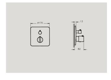
A42292 Diverter, 3-way, exposed part (must be used in conjunction with V-Box A42262) £149° Rec. Minimum pressure: 1.0 bar
