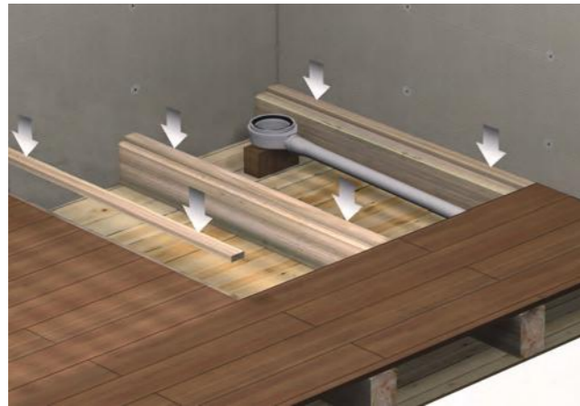
3. Fix timber supports in between joists - these should be fixed low enough to bring your timber panels to the top of the joist.
