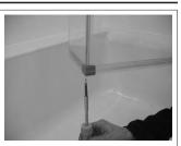
**TIP** Hold the grommet still and finger-tighten the screw only.
