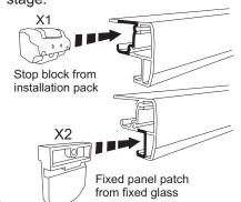
To help with assembly insert the rails into end wraps as shown. The rails are handed, the fixed panel end can be identified by the pre drilled hole at the end. These instructions show a **Right Hand Entry**
