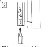
Slide the main height adjuster block into the base of the wall post, it will "Click" when engaged
