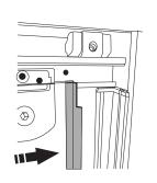
Ensure the lip on the rigid seal locates into the extrusion over it's full length
