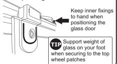
Adjust the hanging of the door so that the closing edge of the glass meets the closing seal evenly over it's entire height. Gain access to screw "A" by removing the top patch cover.
