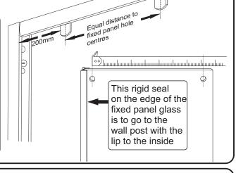
Carefully lift fixed glass panel into the enclosure and secure to fixed panel patches. Make sure you have the 4mm Allen key & inner patch covers to hand. Ensure the rigid seal is to the wall post with the Life Shield treated surface to the inside.
