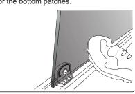
Re-fit the extrusions by reversing the procedure in stage "8" Slide fixed panel back to the fixed side wall post, ensure lip of seal fully locates into the groove in the extrusion. Once secured ensure all allen screws are fully tightened.
