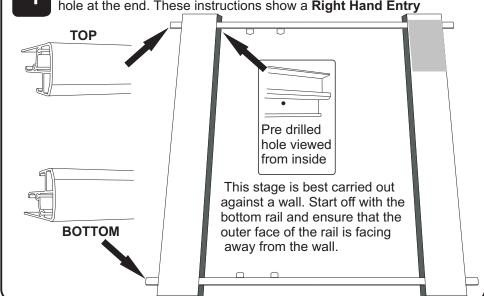
Identify both wall posts. The wall post with the plastic flipper seal as shown will be the opening side of the enclosure, the one without the seal will be the fixed panel side. Please ensure that the wall post without the flipper seal is to go to the end of the rails with the pre drilled hole as shown in stage 4.
