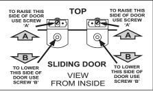
Roller bearing adjustment- using screwdriver, loosen screw (do not remove), reposition in slot and re-tighten.
