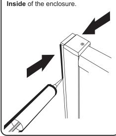
Silicone seal the enclosure to the tray on the outside only You should also seal the joint as shown.
