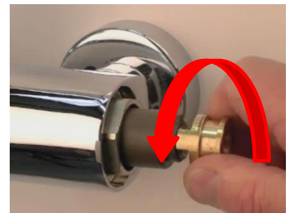
6. If the pre-set temperature is too cold, turn the Temperature Stop lug towards the hot and wait approx. 10 seconds.
