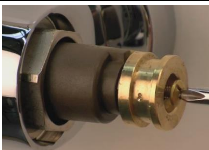
7. Once the Shower is set to the desired temperature, relocate the Temperature Stop Lug onto the Cartridge Spline, ensuring that the Brass Pin is against the Temperature Stop Point of the Temperature Cartridge Cap, and secure with the X-head screw. (This prevents the temperature from exceeding 43°C).
