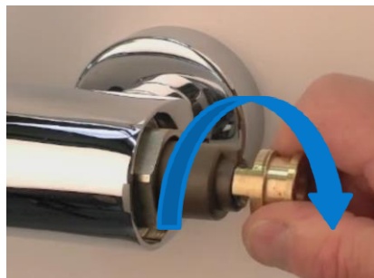
5. If the pre-set temperature is too hot, turn the Temperature Stop Lug towards the cold (clockwise) and wait approx. 10 seconds.
