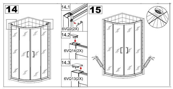
14.Attach the concealed profile 6VQ2 on both side of wall profile. Put profile cap 6VQ14 on top of vertical profile. Put profile cap 6VQ13 on top of wall profile.
