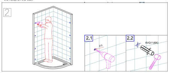
2. Before starting to drill, please check for any hidden electrical cables or pipe work. Drill the holes (( \$6mm) according to the marks and insert the wall plugs(6VQ11) into the holes
