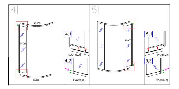
4.Insert fixing part 6VQ15 into the top and bottom rail profile like step 4.1 shows on fixed panel side. Put rail profile 6VQ6 on top and bottom of fixing panel 6VQ3. Fix top and bottom rail profile with vertical profile with screw 6VQ10
