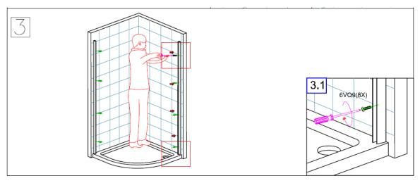
3. Fix wall profile on the wall with screw 6VQ9...
