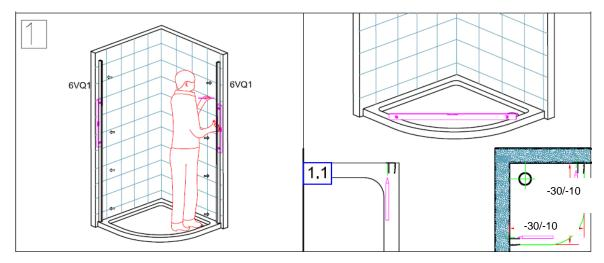
1.Ensure the tray is level with the spirit level and ensure the tray is also correctly installed and sealed as per the manufacturers installation instructions .Put the wall profiles (6VQ1) against the wall, ensuring the distance between the profile and the wall is correct. Adjust the profile to make sure it is vertical by using a spirit level. Mark the holes on the wall.
