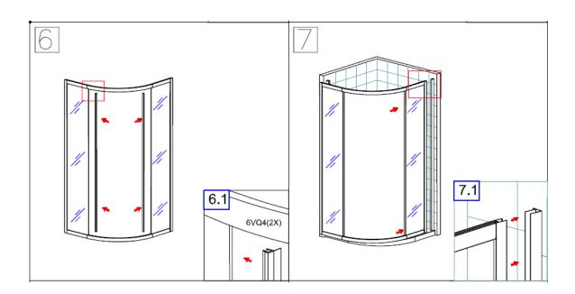
6.Apply vertical seal 6VQ4 on the edge of fixed panel 6VQ3.
