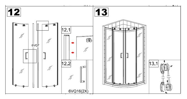
12. Apply magnetic seal 6VQ7 on the sliding door. Mount handle 6VQ16 on the sliding panel.
