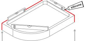
Ensure the shower tray is level in all directions and is properly sealed to the wall. The wall must be tiled down to the top edge of the tray. **Do not angle out bottom tile**.
