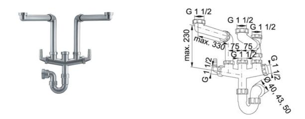
For 1.5 and double bowl sinks. Franke Siphon Plumbing Kits are designed to assist in optimising the underside of the cabinet space and in many cases provided for better utilisation of under-sink storage. Siphon Plumbing Kits have a manifold with an incline and an air vent for faster water disposal, together with a unique Waste Disposal Unit connector on all three models. Made of rigid grey polypropylene, these plumbing kits are the hygienic solution to a Franke sink waste system.
