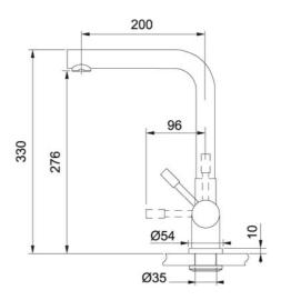
The Minerva Mondial 3-in-1 tap provides hot, cold and 100°C boiling water. Safety is assured with a two-step safety handle, while fully insulated spout and handle ensures that they both stay cool to the touch. Discreet and suitable for almost any kitchen, the horizontal heating tank sits neatly behind a standard 150mm cabinet plinth, freeing up much-needed cupboard space.
