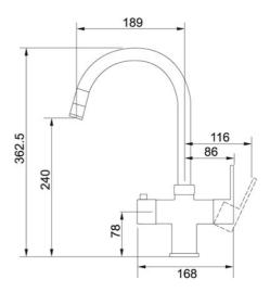
The Minerva Original 3-in-1 tap provides hot, cold and 100°C boiling water. Safety is assured with a two-step safety handle, while fully insulated spout and handle ensures that they both stay cool to the touch. Discreet and suitable for almost any kitchen, the horizontal heating tank sits neatly behind a standard 150mm cabinet plinth, freeing up much-needed cupboard space. The boiling water control can be positioned on the left or right side.
