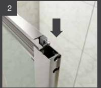
Slot the horizontal profile and screws into upright using guide channel until flush.
