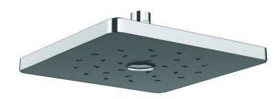
CONSTRUCTION: Brass & ABS SUPPLY: Suitable for all plumbing systems INLET CONNECTIONS: 1/2" BSP WORKING PRESSURES: 0.35 - 5.0 bar CARTRIDGE/VALVE TYPE:N/A
